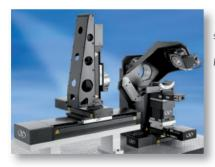
Sensor calibration bench for car-safety systems in automotive industry.
