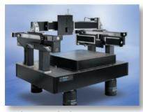
▲ Vibrometer test bench: 3-axis system used at the LCPC (Roads and Bridges laboratory) to measure the density of large concrete blocks. A shock is created in one point with an explosion, the resulting vibrations are measured in another point for analysis of the concrete density.
