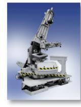
X-ray diffractometers are full custom and turnkey systems used to study the structure and properties of materials. Over 30 diffractometer systems in synchrotrons all over the world serve the scientific community in a large variety of application fields.
