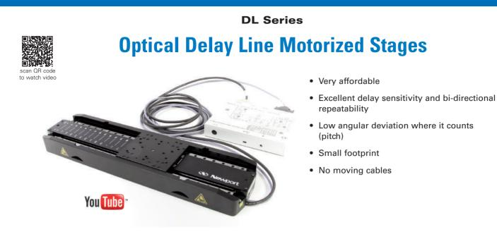
The Delay Line family of affordable linear motor driven stages is optimized for ultrafast spectroscopy applications that require repeatable and precise delays (0.5fs). 3 travel versions and 7 beam kits are available. Delays can be as long as 8.7ns with the 325mm travel version and a 4-pass beam kit. The controller is included with the stage and a user-friendly GUI can be downloaded from the DL family page – making setup quick and easy.
