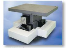
▲ LB Leveling base: High precision 5-axis heavy motorized base used for leveling and positioning a complete optical system. Tripod system, vertical range ±100 mm, tilt ±2.5°. 3000 kg centered load capacity. Optional air-bearing kit.
